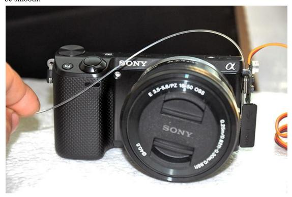
6. Paste the optical fiber cable to the camera infrared receiver window by tape. This finished the installation of the optical fiber cable.
